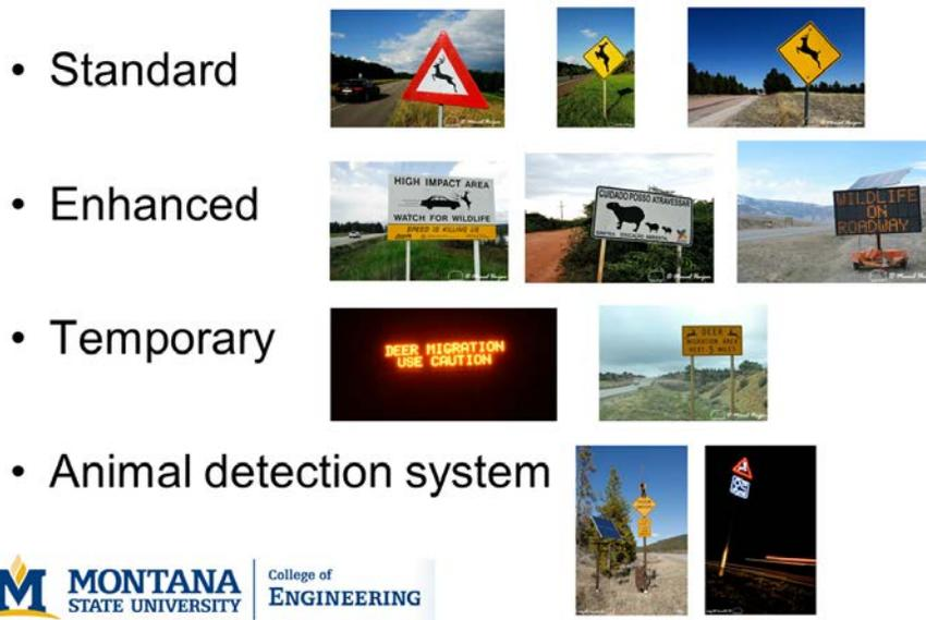
**Figure 3: Four different types of wildlife warning signs.**
