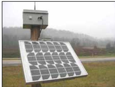
Figure 5.16: A closer view of the box with sensors, battery and the solar panel (Photo: Marcel Huijser, WTI-MSU)
