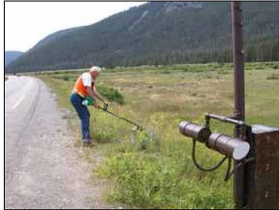
Figure 6.3: Randy Moore mows vegetation in front of one of the sensors to evaluate the effect of high, moving, broad-leafed, and wet vegetation on the occurrence of false positives (Photo: Lloyd N. Salsman/STS)
