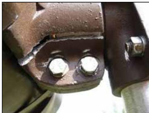
Figure 6.8: The brackets holding the sensors cracked as a result of extreme temperature fluctuations at the MT site
